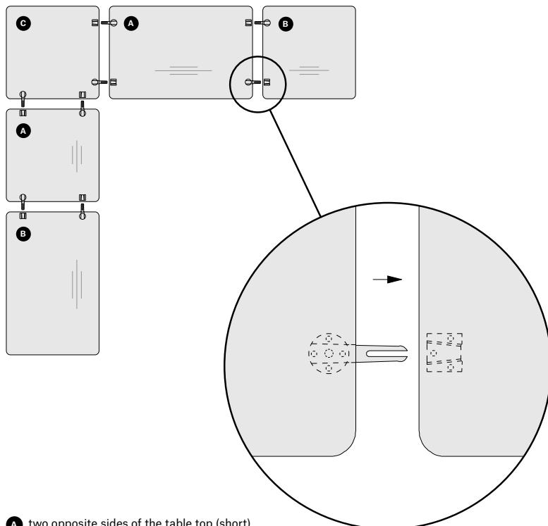
! The lines in the drawing show the direction of the fibres on the table top.
