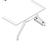
Clips for holding the plastic cables, screwed to the frame leg, detachable cover made of sheet steel coated in signal white, black with a textured matte finish or dark gray with a textured matte finish. Retrofittable on request.
